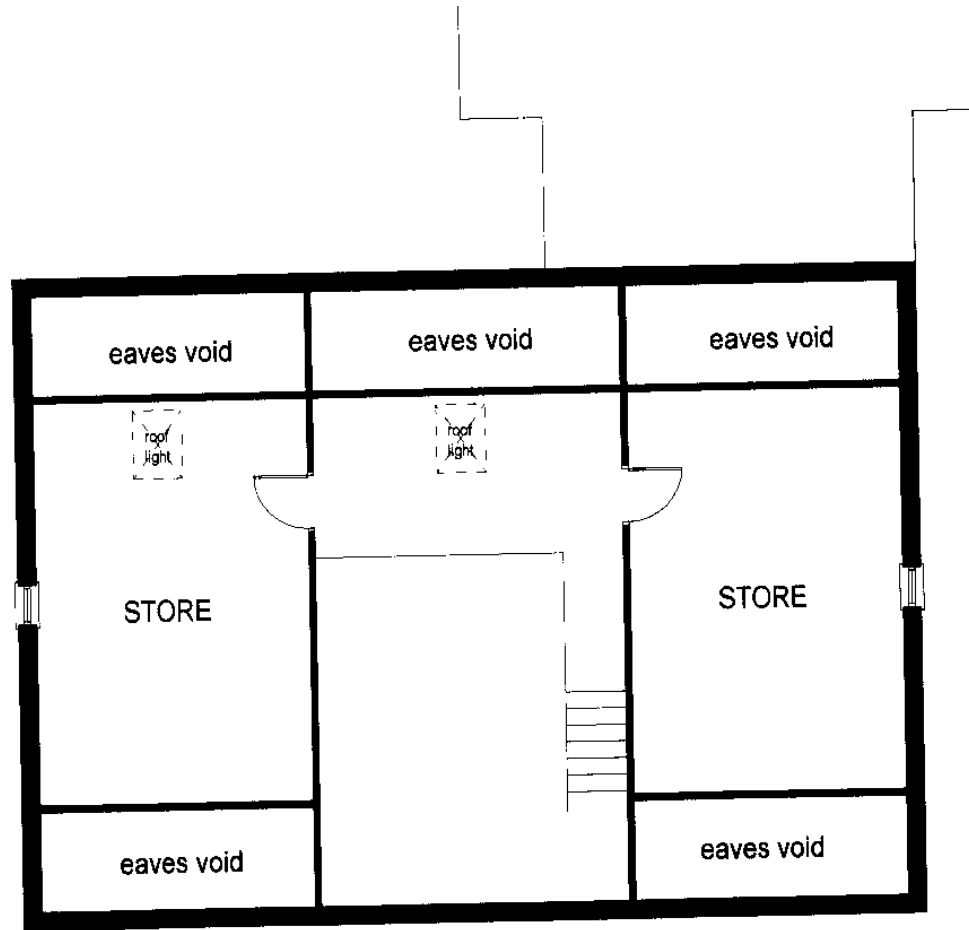
Dwelling Two - Proposed Attic Floor Plan ( scale 1:100 )
